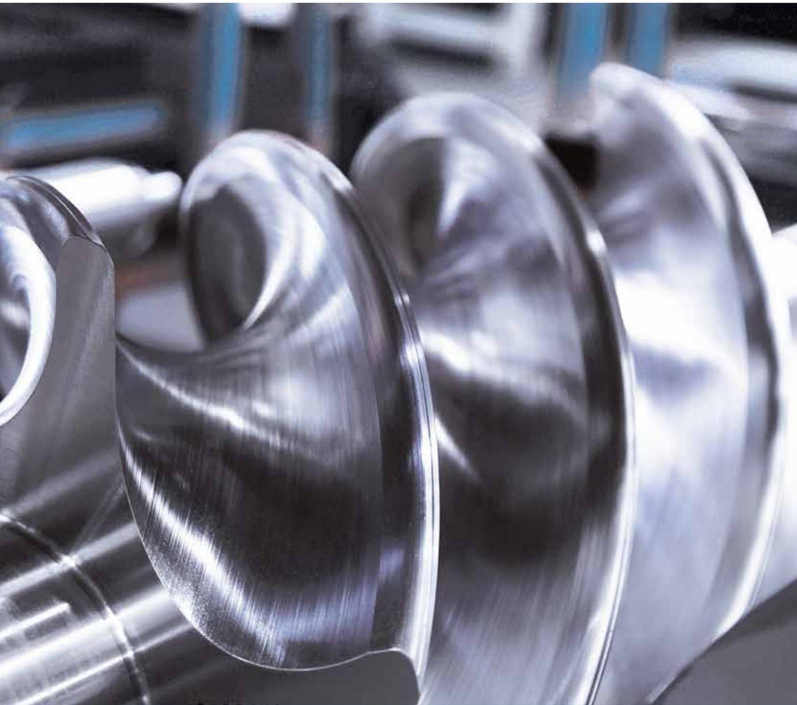
SPECIAL ROTOR PROFILES CHARACTERISE THE SCREW COMPRESSORS MADE BY AERZEN. AND ENSURE THE DECISIVE PERFORMANCE PLUS IN NEGATIVE AND POSITIVE PRESSURE.
