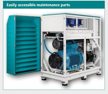
The maintenance parts are easily accessible thanks to removable doors and hinged rear duct silencer. In order to access larger components like motor or air end, the longitudinal bracing can be removed. The separate switch cabinet ensures access to the electrical components.
