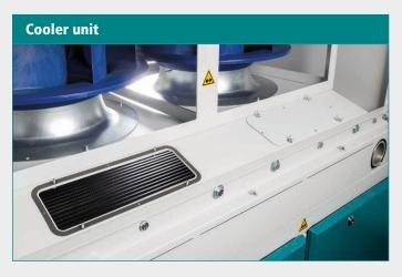
The horizontally mounted cooler can be cleaned by cleaning lids. Alternatively the cooler can be pulled out like a drawer for the purpose of cleaning. Thanks to well dimensioned after coolers for oil and compressed air as well as the integrated oil temperature control, the compressors run reliably even at high ambient temperatures.
