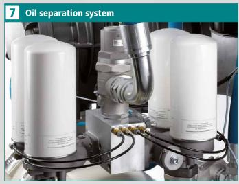
Compressors up to 160 kW are equipped with external separators which can be changed in a simple spin-off/spin-on process. Larger units have an internal separator cartridge. Due to the excellent separation efficiency of the system as a whole, the compressors can be used in the pressure range of 5.0 to 15.0 bar. Special pressures on request.
