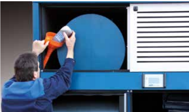
Easy filling of the compressor with lube oil.
