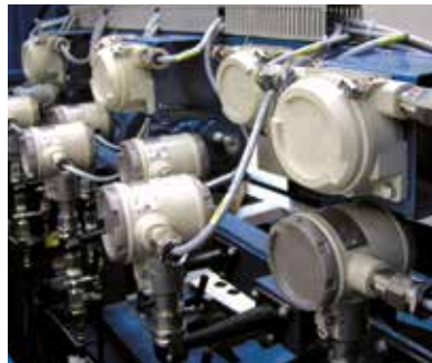
Pressure and temperature transmitter for monitoring the operating data of an argon compressor
